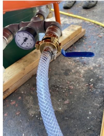
6. Shut the inlet and the mains taps once the juice has stopped flowing. Allow the juice to stop flowing completely. Remove the spray protection hood (if used). **DO NOT** open the press yet.
